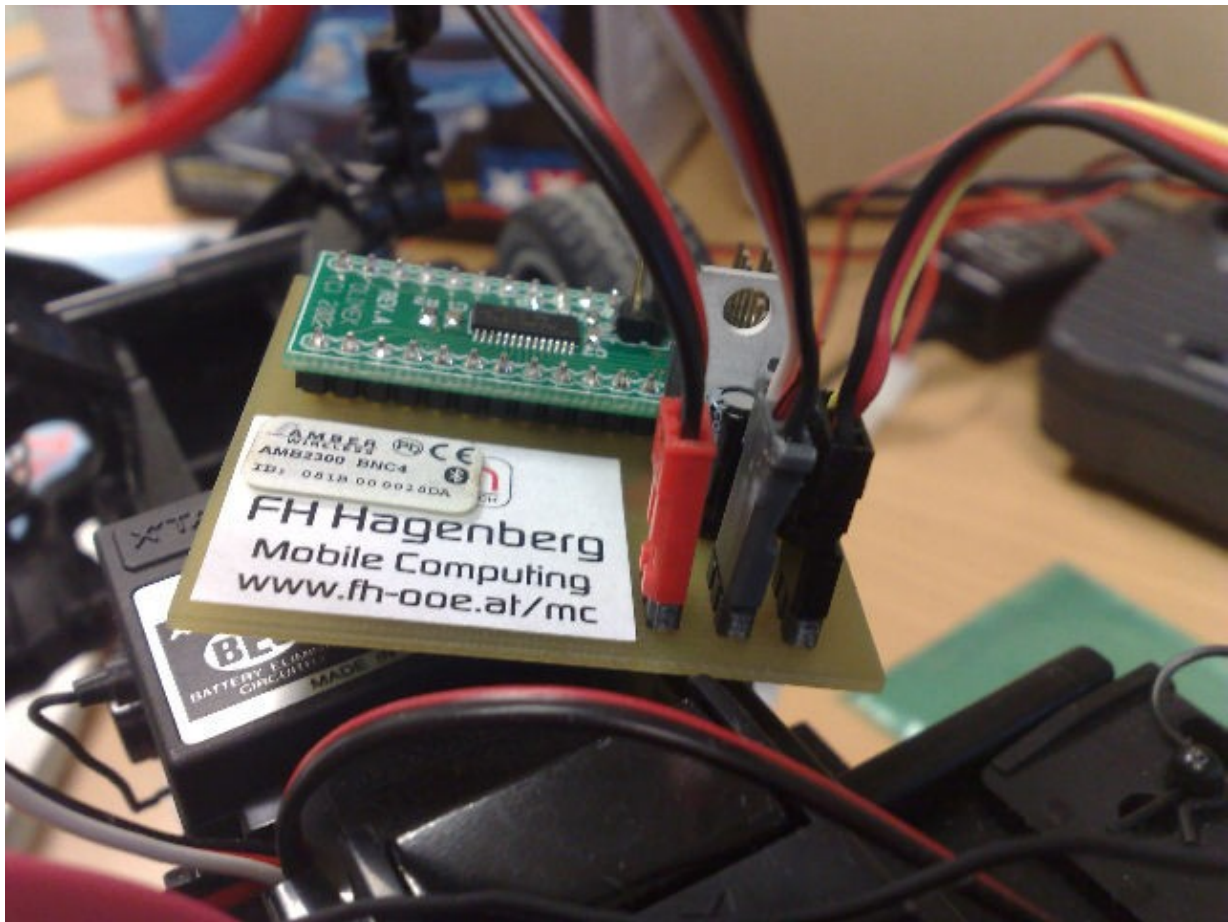
Figure 2: The Bluetooth module connected to the car
