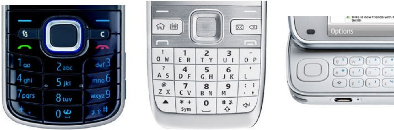
Figure 1: ITU-T keypad in Nokia 6220 classic, half-QWERTY keyboard in Nokia E55 and mini-QWERTY keyboard in Nokia N97
